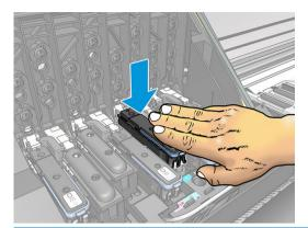
**CAUTION:** You might feel some resistance when installing the new printhead, so you need to press it down firmly but smoothly. You should hear a beep and see confirmation on the front-panel display that the printhead has been inserted.
