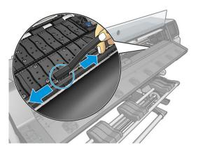
With the same dry brush, remove dry, loosened ink deposits from the platen surface.
