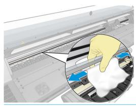
**A** CAUTION: While cleaning, be careful not to damage the plastic encoder strip located on top of the rod.
