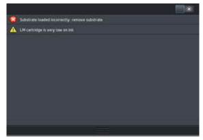
Clicking an alert opens the application that could help to resolve it. Firmware update advice is dismissed when entering the Printer application. Once dismissed, there won't be any reminder later on about the same advice (in the case of firmware updates, a new notification appears when there a new firmware release becomes available).
