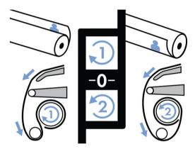
13. Press the button on the front panel to advance the substrate, creating a loop.
