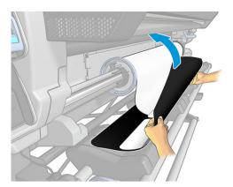
**6.** Load the substrate manually, see <u>Assisted manual load on page 64</u>.
