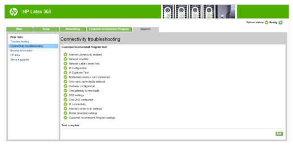
If the test completes successfully, configuration is complete and you can proceed to any other Embedded Web Server page, or close the browser window. If the test fails, follow the instructions to try to identify and fix the problem.
