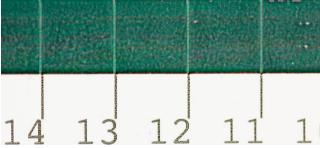
When you have made notes on each row, enter the correction values into the front panel or the Embedded Web Server.
