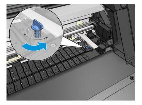
Remove both parts of the platen in the same way. 2.
