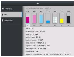
For more details about any particular ink cartridge, press the rectangle representing that cartridge. The following information is shown.
