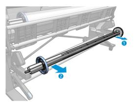
6. For the 335, 365, and 375 printers, lift the lever in each case to remove both of the stops from the take-up reel; they will not be used.
