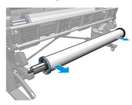
Install the subassembly on the left arm of the tension bar, by moving the arms upwards.
