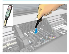
Rub the sponge against the contacts with a *light* force along the entire depth of the flex connector, inserting the wiper as far as allowed by the mechanical stop on the tool.
