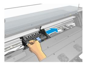
5. Lift the substrate pinch lever as far up as it will go.
