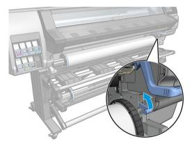
5. Remove the spindle from the printer, pulling out the right end on the right side of the printer first.
