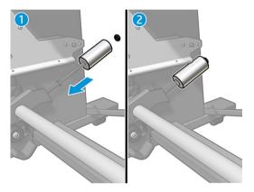
For a 64-inch printer: Keep the weights at the furthest position from the tension bar, to provide maximum counterweight torque.
