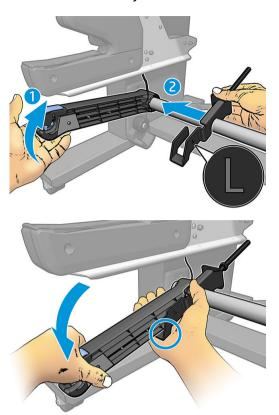
Install the subassembly on the right arm of the tension bar, by moving the arms upwards.
