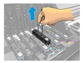
**9.** Gently pull the blue handle upward until the printhead is released from the carriage.
