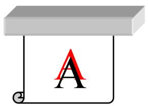
If the colors are misaligned in any direction, the printheads may be misaligned. This is likely if you have not aligned the printheads for a long time, or if there has been a substrate jam. Align the printheads if necessary (see Align the printheads on page 133). You can check whether it is necessary by printing the printhead alignment status plot (see 3. Printhead alignment status plot on page 111).
