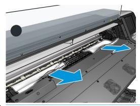
CAUTION: Try to avoid pulling the substrate out through the input path, because this reverses the normal direction of movement, and could damage printer parts.
