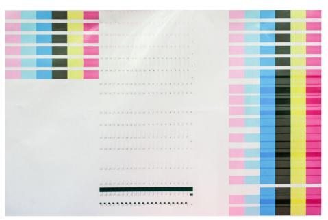
The printer prints 16 rows labelled from A to P. Inspect the print and write down the number of the straightest line in each row (for example, A:9).
