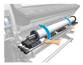
If you regularly use different substrates, you can change rolls more quickly if you pre-load rolls of different substrates on different spindles. Extra spindles are available for purchase.
