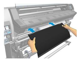
Follow the same method to re-install the platen when required. Attach the velcro to the back of the output platen until tight.
