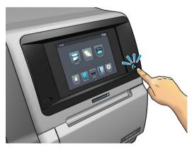
When you turn off the printer this way, the printheads are automatically stored with the maintenance cartridge, which prevents them from drying out.
