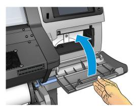
NOTE: Before it can resume printing, the printer needs all the ink cartridges, printheads, and maintenance cartridge to be installed, and the printer window and maintenance cartridge door to be closed.
