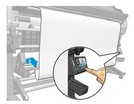
**15.** Press the button on the front panel to advance the substrate again.
