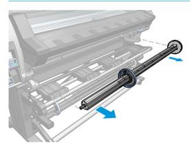
The spindle has a stop at each end to keep the roll in position. Remove the blue stop at the left end to mount a new roll (the stop at the other end of a 76 mm (3 in) diameter spindle can also be removed, if you wish). The stop slides along the spindle to hold rolls of different widths.
