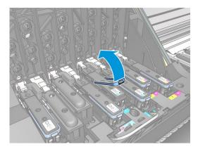
8. Using the blue handle, gently disengage the printhead.
