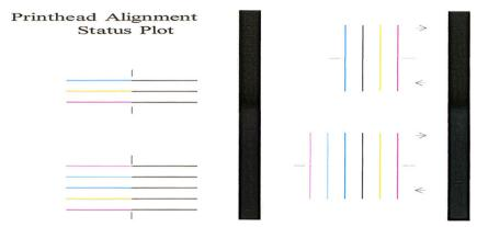
Bear in mind that small misalignments may not cause any print-quality defects. The printing process is designed to hide the effects of small amounts of misalignment. The reference scale can be used to quantify the amount of misalignment; errors below 4/600 inch are unlikely to cause print-quality defects.
