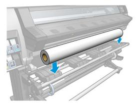
7. Slide the spindle into the roll.
