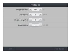
To change substrate advance calibration while printing (in case of banding): press Adjustments > Adjust substrate advance. The changes that you make take effect immediately, but they are not saved for the next job. See also <u>Substrate advance adjustment while printing on page 113</u>.
