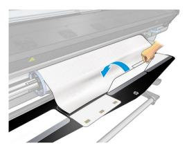
5. Lift the loading accessory and the leading edge of the substrate together.
