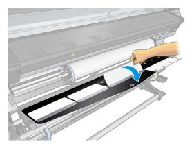
3. Pull some of the substrate from the roll and put the leading edge on the loading accessory.
