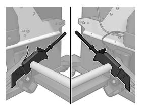
Install the weight at the end of the nut for most substrates. In some cases, you can move the weight forward to reduce the front tension for a particular substrate.
