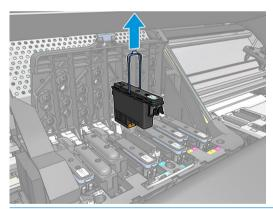
CAUTION: If you want to preserve the old printhead for later use, reinstall the cap and plug, but never install a clear optimizer cap or white plug on a non-optimizer printhead. Optimizer printheads have clear caps and white plugs, while the other printheads have orange caps and plugs. Installing the wrong cap and plug can cause irrecoverable printhead damage.
