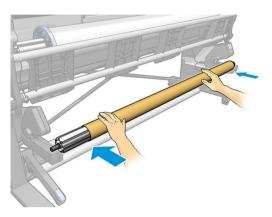
Advance the substrate by pressing the **Move substrate** button on the front panel. Make sure that the substrate passes in front of the loading table.
