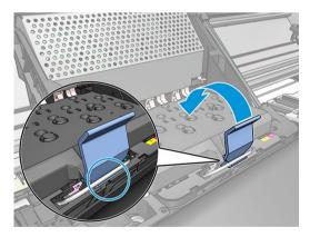
Lower the latch to rest on the carriage cover.
