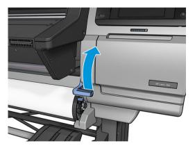
**6.** Carefully remove as much as possible of the jammed substrate from the top of the printer. Cut the substrate if necessary.
