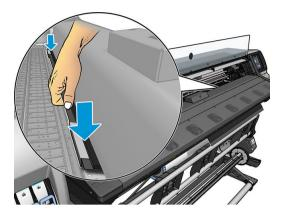
**d.** Make sure the platen protector is well positioned and straight.
