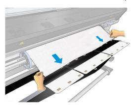
**4.** Flip the white flaps back to cover the leading edge of the substrate. The black patches are magnetic and grip the substrate.
