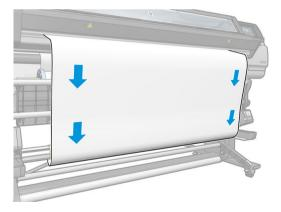
14. Press the blue arrow on the take-up reel motor to rotate the reel one full turn. This will help to support the weight of the tension bar.
