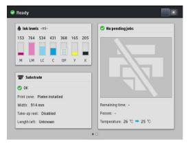
The front panel has a large central area to display dynamic information and icons. On the left and right sides you can see up to six fixed icons at different times. Normally they are not all displayed at the same time.
