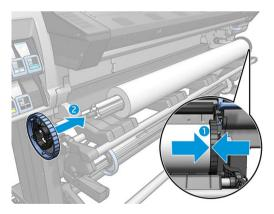
10. Lock the blue stop when it is in contact with the substrate.
