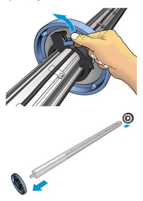
7. Load the core onto the take-up reel. The core should be at least as wide as the substrate.
