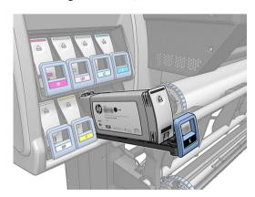
Lift the cartridge out of its drawer.
