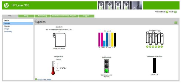
The Supplies page shows you the status of the loaded substrate, the ink cartridges, the printheads, the heater, and the maintenance cartridge.
