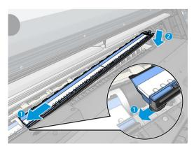
**4.** Ensure that the locks are locked and that there is no obstruction in the printing path.
