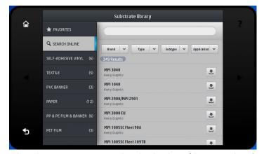
When the printer is connected to the database (this may take a few seconds), a list of all available substrate presets for your printer model is displayed. You can browse the list by scrolling it, and get details on any preset by pressing its name. Besides browsing, there are two additional ways to look for presets: free-text search and filters.
