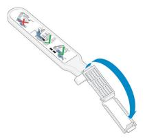
Load the sponge by positioning the sponge on the face of the carriage interconnect wiper with the shorter tab in the locating slot.
