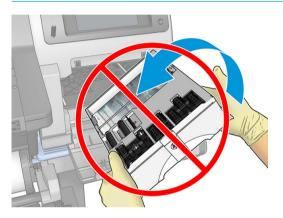
5. Remove the plastic cover from the new maintenance cartridge.
