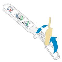
Open the printhead carriage latch and extract the printhead that is causing the problem, as indicated on the front panel. See Replace a printhead on page 135.
