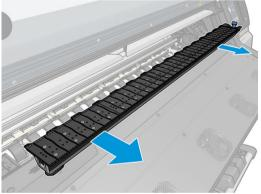
Place the two parts of the ink collector into the printer. 3.
