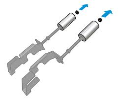
Remove the tension bar.
