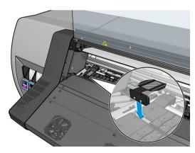
2. Slide the edge holder into its correct position.
