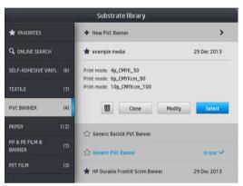
If you delete a preset, you will lose the reference to that substrate in the usage and accounting information. Instead of the name of the substrate, from that moment on you will see "Deleted substrate" in the usage and accounting information.
