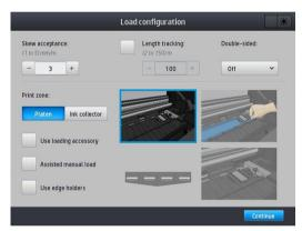
You can alternatively begin at step 2, in which case the load configuration screen will appear with this checkbox checked after you lift the pinch lever. Press **Continue** before taking the next step.
