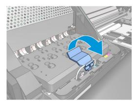
Lift up the cover. This provides access to the printheads.
