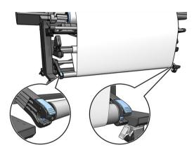
**19.** Use the winding-direction switch on the take-up reel motor to select the winding direction. Setting **1** winds the substrate so that the printed image faces in. Setting **2** winds the substrate so that the printed image faces out.
