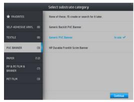
Generic presets are each designed for a whole substrate category, rather than for a particular substrate type. They cannot be edited, erased, saved, color-calibrated or ICC profiled; but they can be cloned. Therefore, if you would like to modify a generic preset in any way, you should first clone it and then work on the clone, which is fully editable.
