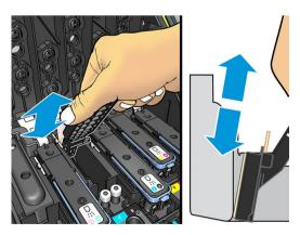
Using the same sponge, clean the lower strip of electrical contacts on the printhead (unless the printhead is new). Avoid touching the upper set of electrical contacts.
