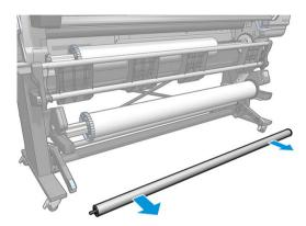
Remove the take-up reel to facilitate the installation of the new arms with counterweights.
