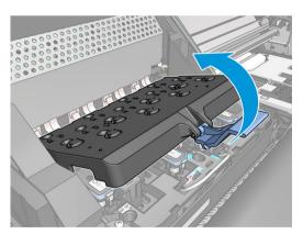
7. To remove a printhead, lift up the blue handle.
