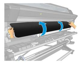
7. The loading accessory passes through the printer's substrate path with the substrate.
