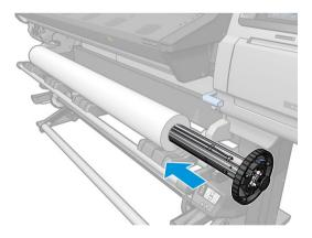
8. The right stop of the 76 mm (3 in) diameter spindle has two positions: one for rolls of the printer's maximum width, and another for narrower rolls. Remember to use the second position for narrower rolls, which improves the curing process and allows higher printing speeds.
