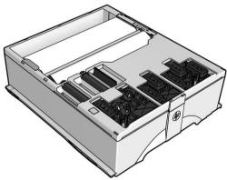
The cartridge contains a roll of cloth, which is used to clean the printheads. You are notified when 92% of the roll has been used, after which the cartridge should continue to function for about another 140 m² (1500 ft²) of printed area. A new roll lasts for about 1850 m² (20000 ft²) of printed area.
