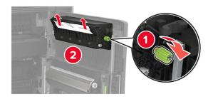
3 Open the standard trays, and then remove the jammed paper.Note: Make sure that all paper fragments are removed.
