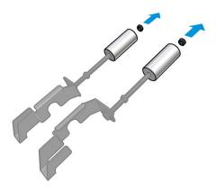
2. Remove the tension bar.
