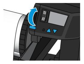
8. Remove the take-up reel from the printer, pulling out the end on the right side of the printer first.
