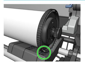
9. Put the blue stop on to the upper end of the spindle, and push it towards the end of the roll.
