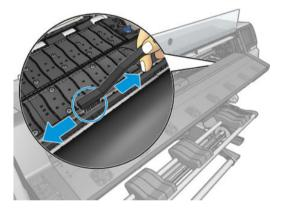
3. With the same dry brush, remove dry, loosened ink deposits from the platen surface.
