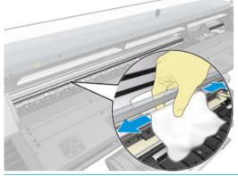
**<u>A</u> CAUTION:** While cleaning, be careful not to damage the plastic encoder strip located on top of the rod.
