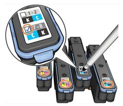
Printheads use shipping fluid, which must be purged when a printhead is first inserted. For further information see <u>Insert a printhead on page 144</u>.
