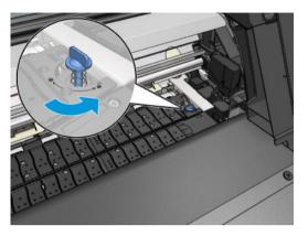
2. Remove both parts of the platen in the same way.
