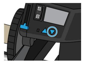
**15.** Tap the button on the front panel to advance the substrate again.
