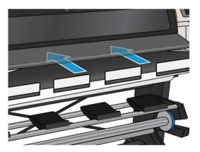
6. The loading accessory passes through the printer's substrate path with the substrate.
