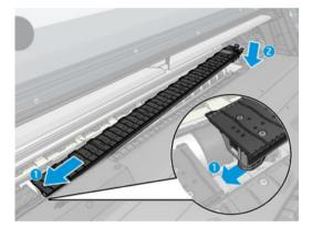
4. Repeat with the platen module or ink collector on the other side.
