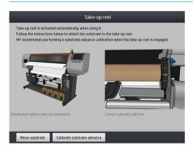
Load a core onto the take-up reel. Insert it first onto the right hub. 2.
