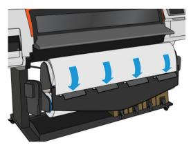
5. Flip the white flaps back to cover the substrate's leading edge. The black patches are magnetic and grip the substrate.
