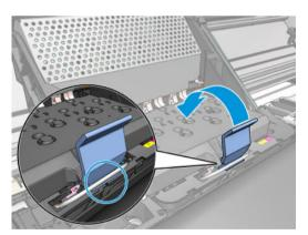
8. Lower the latch to rest on the carriage cover.
