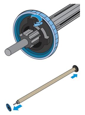
7. Load the core onto the take-up reel. The core should be at least as wide as the substrate.
