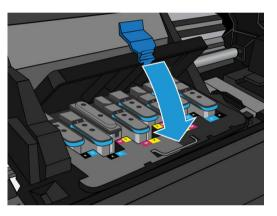
7. Make sure that the end of the latch catches the wire loop on the near side of the carriage.
