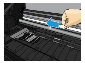
4. Close the window. The carriage moves to the left-hand side of the printer.
