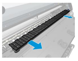
3. With care, smoothly place the two parts of the ink collector into the printer.
