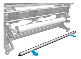
3. Remove the take-up reel to facilitate the installation of the new arms with counterweights.
