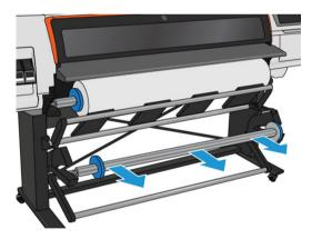
6. Lift the lever in each case to remove both of the stops from the take-up reel; they will not be used.
