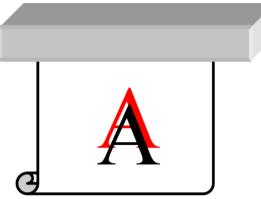
If the colors are misaligned in any direction, the printheads may be misaligned. This is likely if you have not aligned the printheads for a long time, or if there has been a substrate jam. Align the printheads if necessary (see <u>Align the printheads on page 140</u>). You can check whether it is necessary by printing the printhead alignment status plot (see <u>2. Printhead alignment status plot on page 113</u>).
