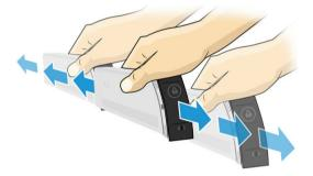
4. Insert the intermediate tank into the drawer.
