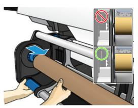
4. Advance the substrate until it reaches the take-up reel core.
