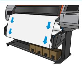
11. The following image shows how the printer looks when it is operating. As substrate is fed from the printer, it drops down to the take-up reel.
