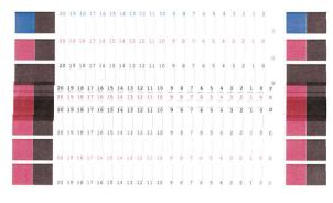
• HP Stitch S500: The printer prints 20 rows labelled from A to T. Inspect the print and write down the number of the straightest line in each row (for example, A:9).
