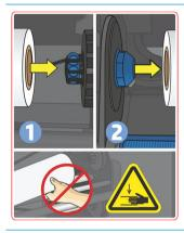
Crush risk. Be careful when loading rolls: your hand could be crushed between the roll and the substrate input structure.
