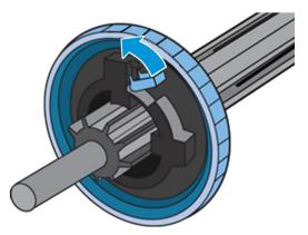
5. Remove the stop from the left end of the spindle.
