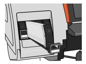
5. Lift the intermediate tank out of its drawer.
