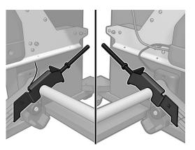
7. Install the weight at the end of the nut for most substrates. In some cases, you can move the weight forward to reduce the front tension for a particular substrate.
