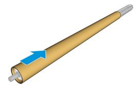
8. Load the take-up reel into the printer by pushing firmly on both ends.
