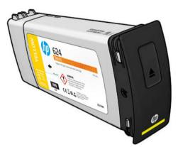
Ink cartridges require no maintenance or cleaning, but must be shaken before installation. Color cartridges should be shaken 6 times; black cartridges should be shaken 30 times.
