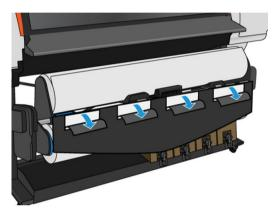
4. Pull some of the substrate from the roll and place the leading edge under loading accessory's magnetized white flaps.
