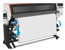
**17.** Carefully insert the tension bar. This is essential: the take-up reel will not function correctly without it.
