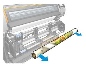
2. Rotate the pivot system so that the input roll is accessible.
