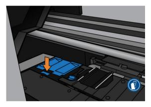
4. Close the window. The cartridge moves to check if there is any mechanical interference. If there is no issue, continue with the following steps. If there is an issue, you are asked to repeat the process and reinsert the ink funnel.
