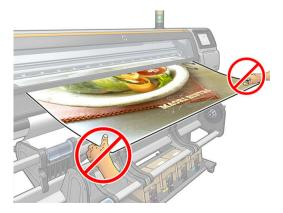
• When printing a series of jobs, do not let the printed substrate obstruct the output path: this can cause severe print-quality defects.
