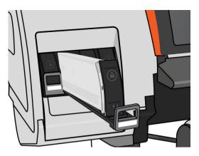
4. Lift the cartridge out of its drawer.
