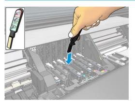
7. Rub the sponge against the contacts with a *light* force along the entire depth of the flex connector, inserting the wiper as far as allowed by the mechanical stop on the tool.
