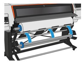
4. Unlock the take-up reel by pushing its lever to the uppermost position.
