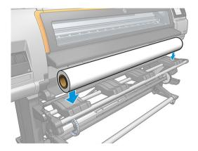
7. Slide the spindle into the roll.
