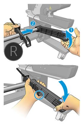
6. Correct the position of the tension bar after installing the arms.
