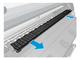
2. Slide the edge holder onto the platen module or ink collector, and adjust its position: on the left, as far to the left as possible; on the right, as far to the right as possible.
