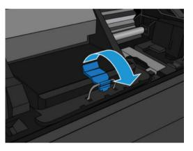
6. Lift up the cover. This provides access to the printheads.
