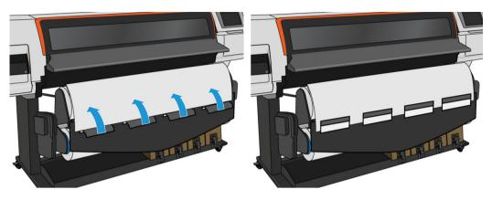
6. Feed the loading accessory into the substrate input.
