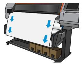
9. Move the blue lever on the take-up reel motor to rotate the reel one full turn.
