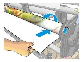
5. Remove the left hub from the roll, resting the roll on the table.
