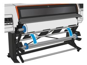
If you regularly use different substrates, you can change rolls more quickly if you pre-load rolls of different substrates on different spindles. Extra spindles are available for purchase.
