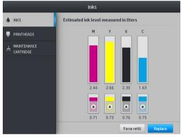
When grayed out, the 3 liter cartridge is refilling and cannot be used.
