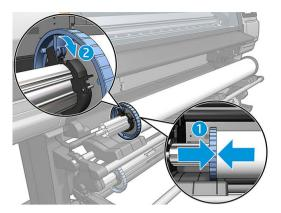
**11.** Insert the spindle carefully into the printer.
