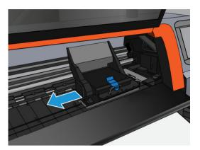
5. The front panel prompts you to reopen the window and clean the right-hand side of the encoder strip (inside the service station). Tap **Continue** when finished.
