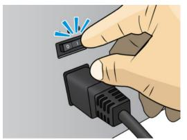
To turn it back on later, use the power switch at the rear. If the printer does not start automatically, press the power button.
