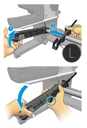
5. Install the subassembly on the right arm of the tension bar, by moving the arms upwards.
