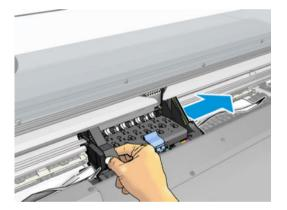
5. Carefully remove as much as possible of the jammed substrate from the top of the printer. Cut the substrate if necessary. The pinchwheels should have lifted to simplify clearing the jam. If this has not happened, restart the printer with the window open to force the pinchwheel movement and the release of the substrate.
