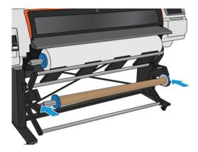
9. Advance the substrate by tapping the **Move substrate** button on the front panel. Make sure that the substrate passes in front of the loading table.
