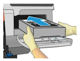
6. Push the maintenance cartridge in until it does not protrude from the slot. You will notice that the printer takes it; do not use excessive force.
