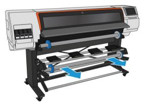
The spindle has a stop at each end to keep the roll in position. Remove the blue stop at the left end to mount a new roll (the stop at the other end of a 76 mm (3 in) diameter spindle can also be removed, if you wish). The stop slides along the spindle to hold rolls of different widths.
