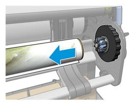
7. Remove the roll from the printer.
