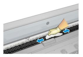
5. Use the damp cloth to remove remaining dry ink deposits from the cutter ramp.
