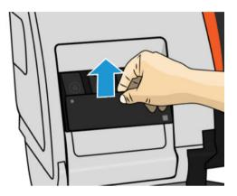
3. Grip the blue tab in front of the intermediate tank that you want to remove, pull the blue tab down and then pull it outwards towards you.
