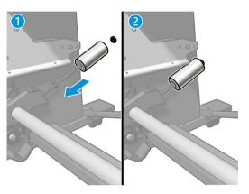
8. Keep the weights at the furthest position from the tension bar, to provide maximum counterweight torque.
