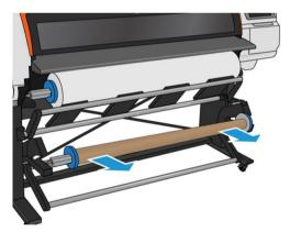
4. Install the subassembly on the left arm of the tension bar, by moving the arms upwards.
