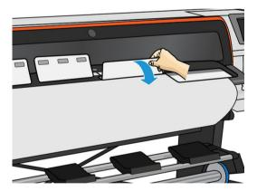
4. Check the **Use loading accessory** box in the Load Configuration screen on the front panel, so that you will have the correct loading sequence, and to set the correct mechanical settings for thin substrates.
