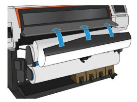
7. The loading accessory passes through the printer's substrate path with the substrate.
