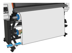
**18**. Fit the tension bar into the supports at either side.
