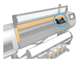
5. Pull up and release the latch on top of the carriage.
