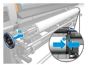
**10.** Lock the blue stop when it is in contact with the substrate.
