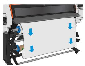
14. Press the blue arrow on the take-up reel motor to rotate the reel one full turn. This will help to support the weight of the tension bar.
