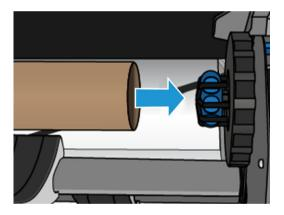
Insert the left hub into the core. Press laterally to ensure that it is tightly inserted. 3.
