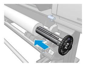
8. The right stop of the 76 mm (3 in) diameter spindle has two positions: one for rolls of the printer's maximum width, and another for narrower rolls. Remember to use the second position for narrower rolls, which allows higher printing speeds.
