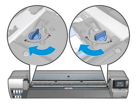
Follow the same method to reinstall the platen when required.
