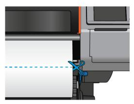
4. While holding the substrate, use the winding button on the take-up reel motor to wind the remainder of the substrate around the take-up reel.
