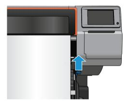
5. Remove the spindle from the printer, pulling out the right end on the right side of the printer first.
