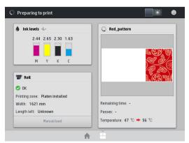
The front panel has a large central area to display dynamic information and icons. On the left and right sides you can see up to four fixed icons at different times. Normally they are not all displayed at the same time.
