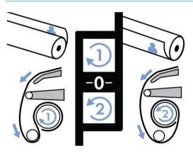
**13.** Tap the button on the front panel to advance the substrate, creating a loop.
