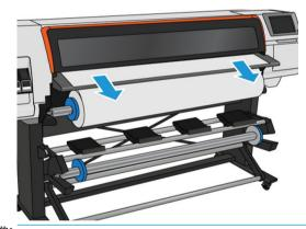
6. Wait until the substrate emerges from the printer, as shown below.
