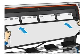
**3.** Flip the white flaps back to cover the leading edge of the substrate. The black patches are magnetic and grip the substrate.
