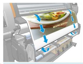
NOTE: If the take-up reel is loaded before printing, recalibrate the substrate-advance sensor for optimal print quality. At the front panel, tap **Take-up reel** > **Calibrate substrate advance**.
