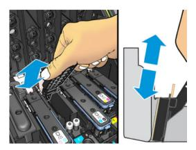
9. Using the same sponge, clean the lower strip of electrical contacts on the printhead (unless the printhead is new). Avoid touching the upper set of electrical contacts.
