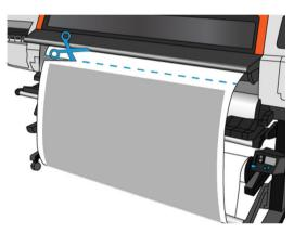
6. While holding the substrate, use the winding button on the take-up reel motor to wind the remainder of the substrate around the take-up reel.
