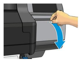
2. The maintenance cartridge has a handle on the front. To remove the cartridge, just slide it out.
