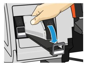
5. Slide the drawer and intermediate tank into the slot until they lock into position.
