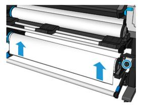
7. Unlock the take-up reel by pushing its lever to the uppermost position.
