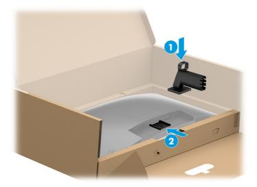
4. Attach the base to the monitor stand (1) and tighten the screw (2).
