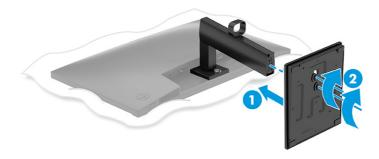
Attach the base to the monitor stand, and then snap the base onto the stand.
