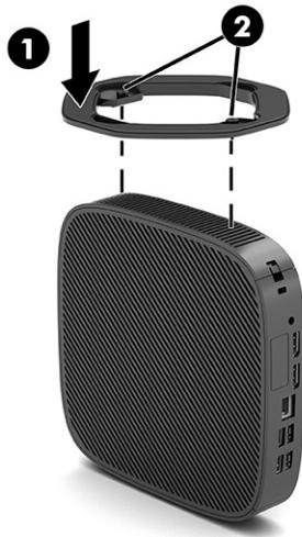
6. **Horizontal orientation:** Attach the stand to the right side of the thin client.
