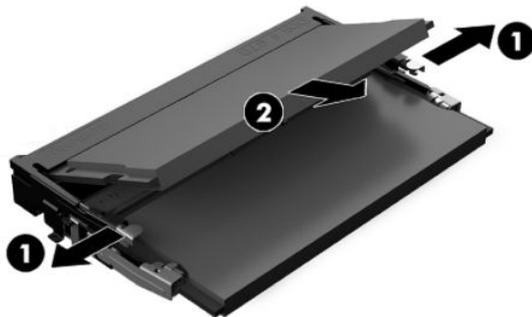
4. Slide the new memory module **(1)** into the socket at approximately a 30° angle, and then press the memory module down **(2)** so that the latches lock it in place.
