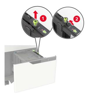
**b** If the A5 length guide is still attached, then remove it. If the guide is not attached, then proceed to <u>step</u> <u>d on page 34</u>.
