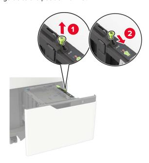
**b** Squeeze and slide the length guide to the position for A5 until it *clicks* into place.
