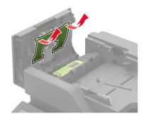
4 Remove the used ADF feed roller.
