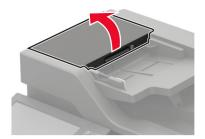
**3** Remove the ADF separator roller cover.
